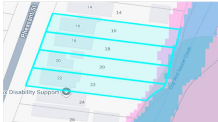
Figure 6: Approximate flood risk areas – 100-year level in blue, probable maximum flood level in pink Source: Weave- CBC Maps
