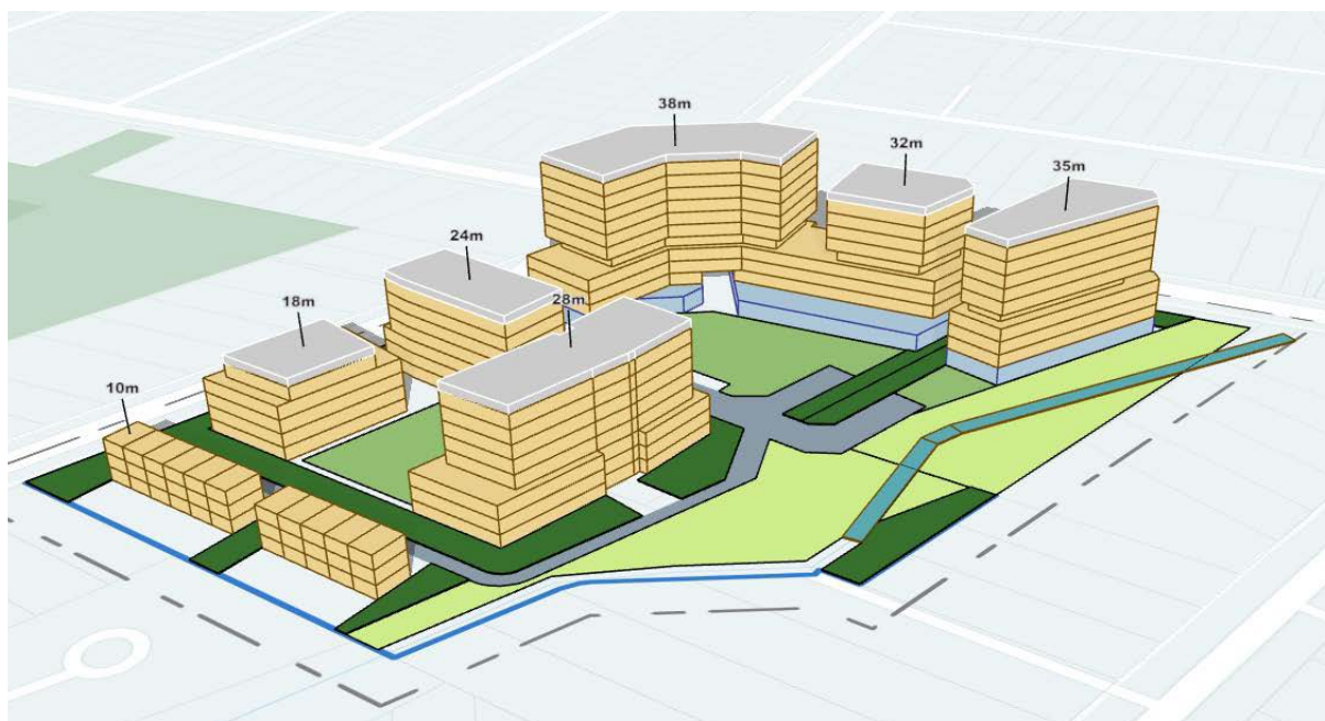
Figure 20: Scenario 3: Council's preferred scenario, viewed from the north west, showing maximum building heights (grey shading on the top of the buildings is a 2m mechanical plant height allowance).
